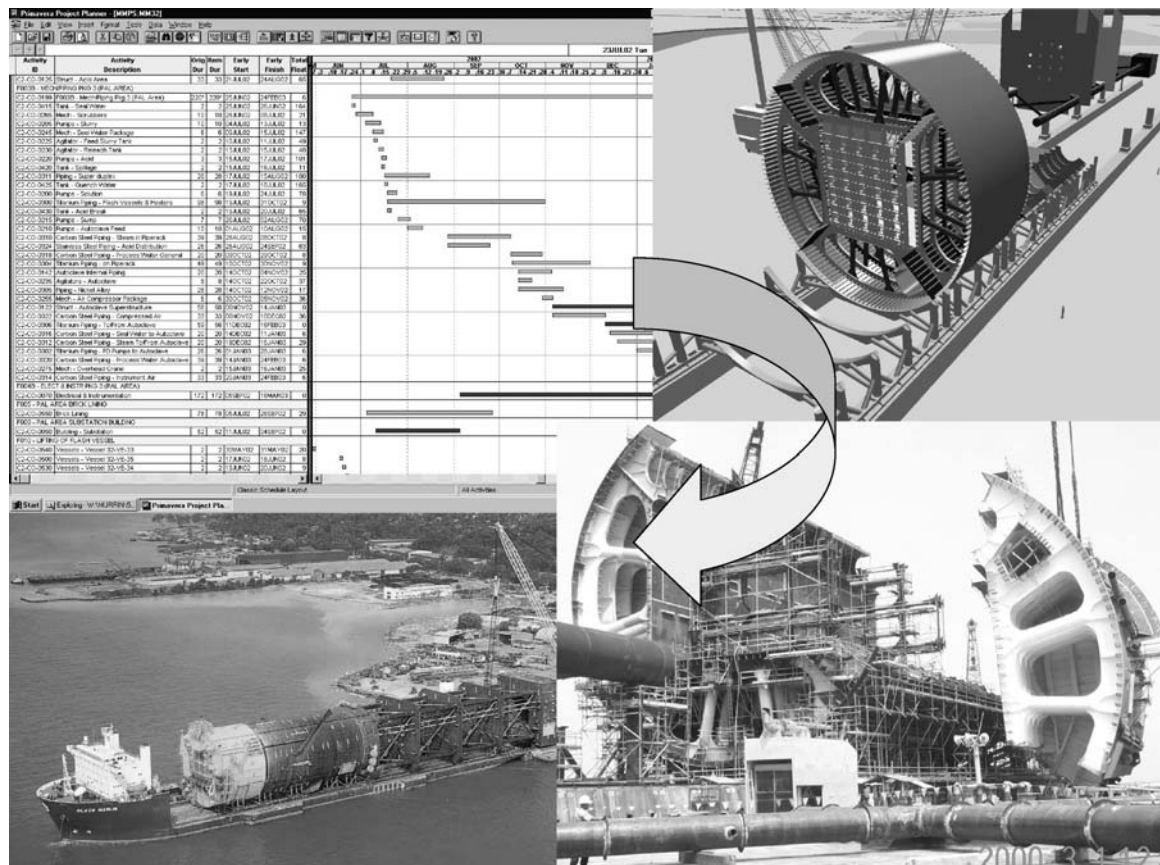
Figure 3: Composite picture showing project planning, 3D-design, fabrication to delivery processes largely driven by databases (pictures and design courtesy of J.Ray McDermott Far East)
