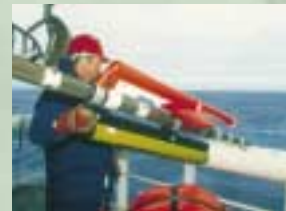
Streamer deployment on the Föhn vessel in the North Sea.
